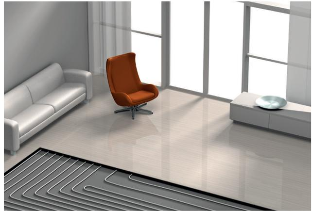
A **Radiant** cooling system operates at warmer temperatures than traditional All-Air cooling systems. Typically, the circulating water only needs to be 6-8°C below the desired indoor air temperature. Once absorbed by the actively cooled surface, heat is removed by water flowing through a hydronic circuit, replacing the warmed water with cooler water. Radiant cooling is most effective at removing direct solar and sensible heat gains.
